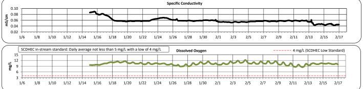
Note: Data gaps appear when the sonde is removed for calibration or when the flow depth is below the sensors
