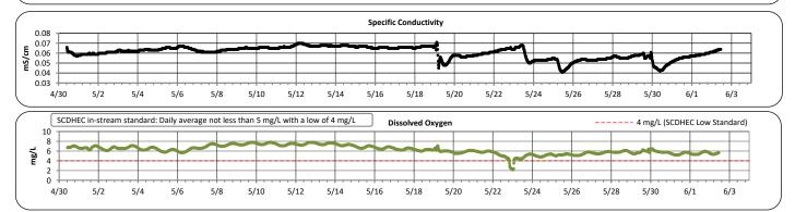
Note: Data gaps appear when the sonde is removed for calibration or when the flow depth is below the sensors
