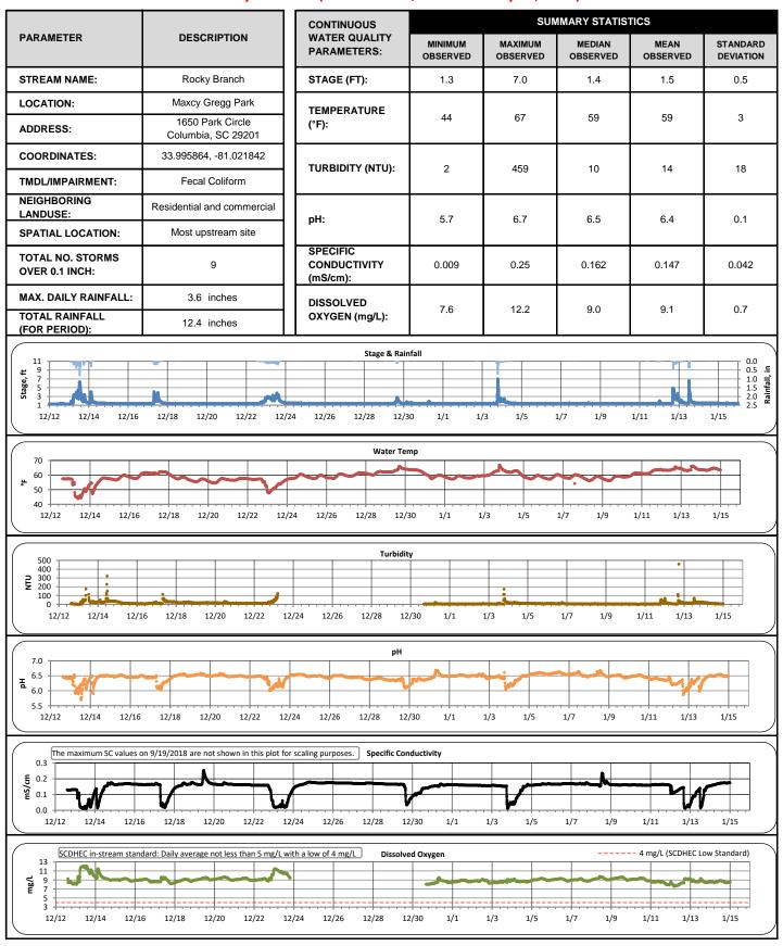
Note: Data gaps appear when the sonde is removed for calibration or when the flow depth is below the sensors
