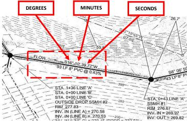
\*The same example can apply for storm drainage with the addition of junction boxes or catch basins\*
