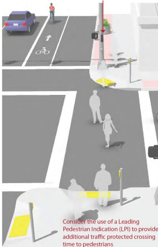
Figure 9-17. Accommodating Pedestrians at Signalized Crossings
