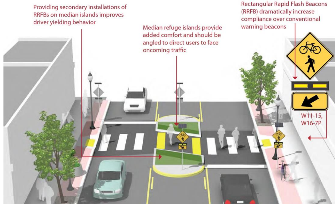
Figure 9-18. Active Warning Beacons (RRFB)
