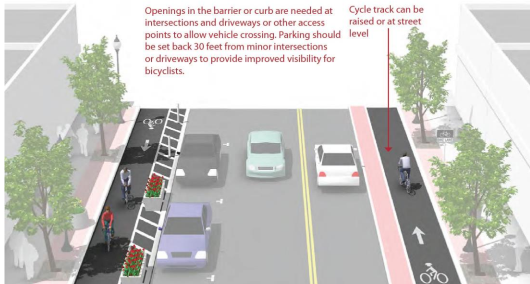
Figure 9-48. Cycle Track Separation And Placement
